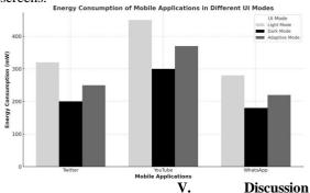
The findings of this study highlight the significant impact of UI color schemes on power consumption in mobile and computing devices. The results indicate that darker UI themes, particularly on OLED-based displays, contribute to measurable energy savings compared to lighter themes. This section interprets these findings, discusses their broader implications, and provides recommendations for UI/UX designers and developers while addressing potential usability concerns.
