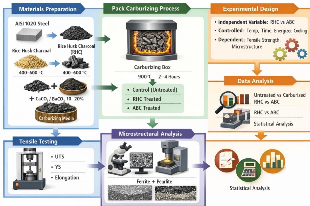
Fig. 1 Experimental Setup for Pack Carburizing Process
