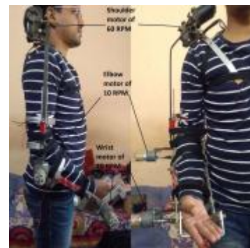
Figure 8: Front view and side view of Exoskeleton arm
