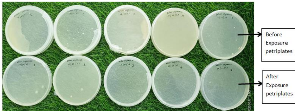
Fig 2: Comparison in reduction of bacteria in Tryptone Soy agar petri dishes of before and after ozonation
