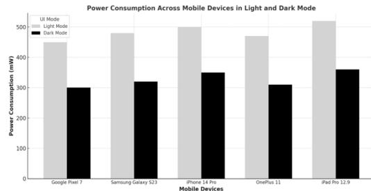
Figure 1: Power Consumption Comparison (Dark vs. Light Mode)
